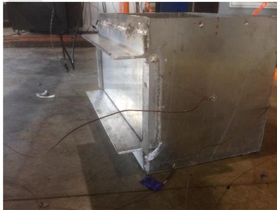
Figure 121. **Aluminum Enclosure with Frame Mounting Flanges**
