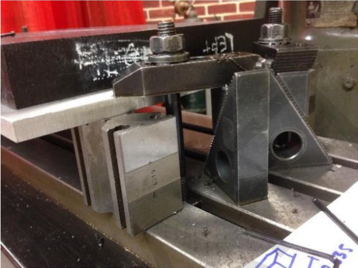
Figure 24. **Material Hold Down for Separator Machining**
