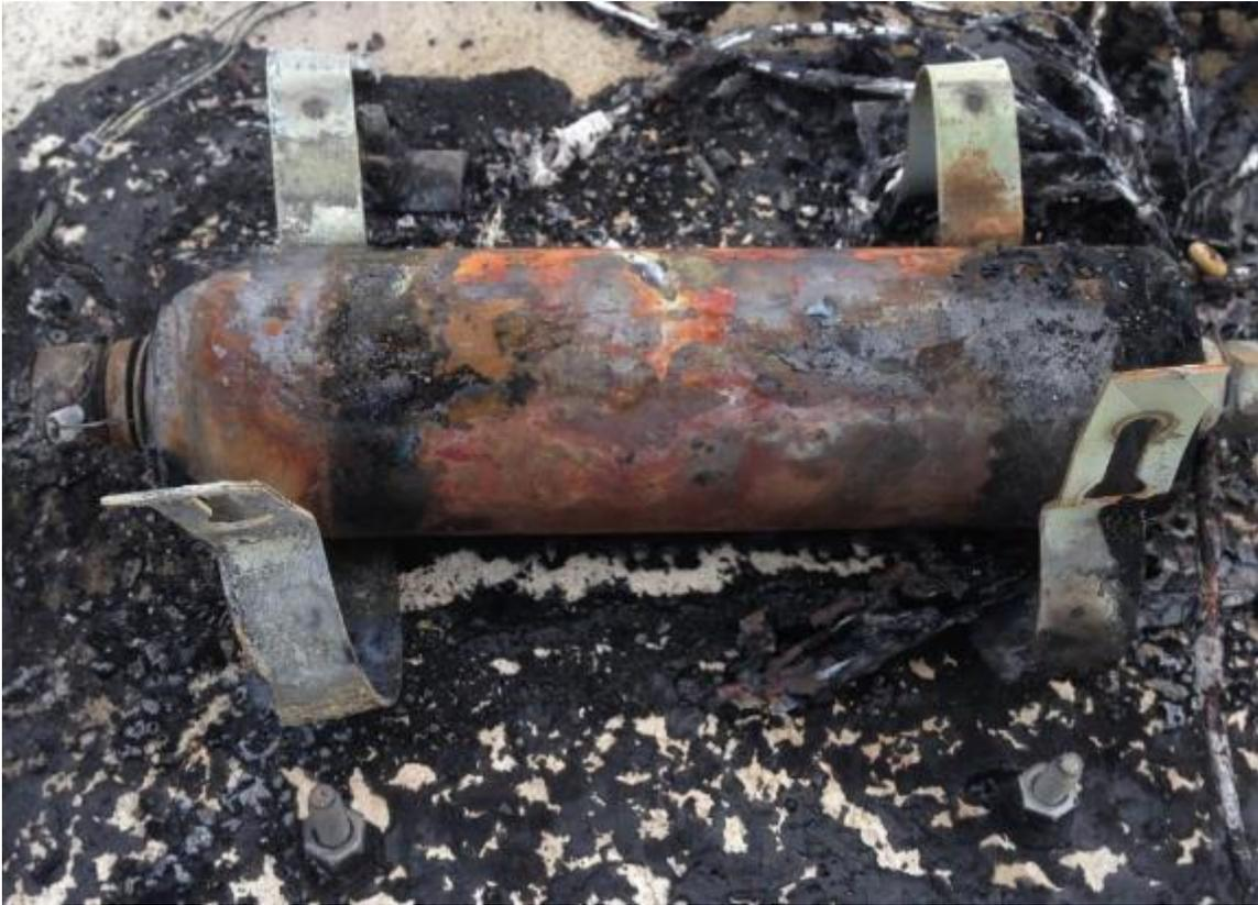
Figure 43. Cell, Hours After Venting Event
