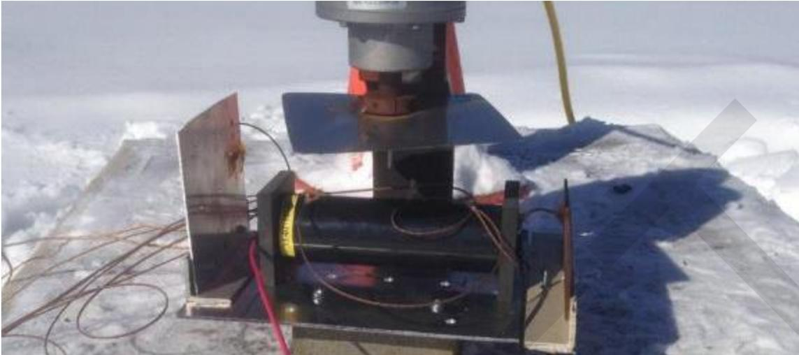
Figure 46. **Acetal Overcharge with Blast Shield Material Test Setup**
