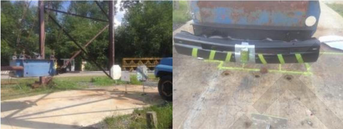
Figure 119. **Pendulum Test Swing Setup**
