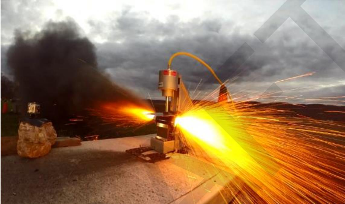
Figure 2. **Single Cell Nail Puncture Test**
