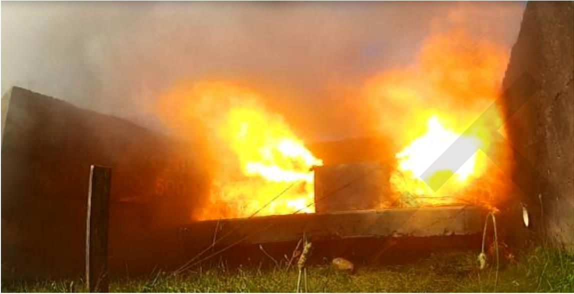
Figure 109. **Battery Pack Venting**
