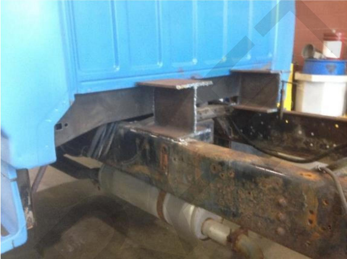
Figure 114. **I Beam Sections Welded to Chassis Frame**
