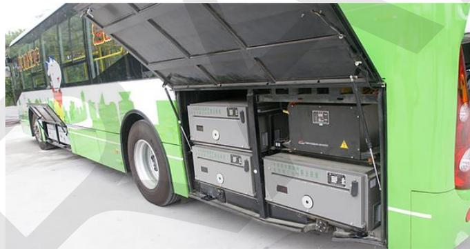
Figure 11. **Battery Packs on the Side of the Bus**
