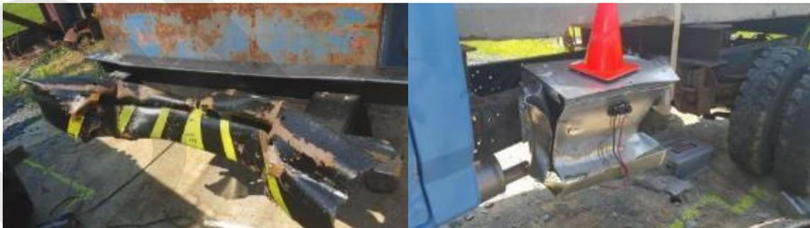
Figure 126. **Deformation of bumper and module enclosure**
