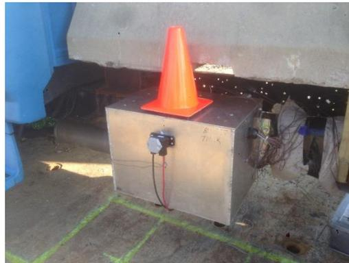
Figure 122. **Battery Module Mounted on Frame with Data Acquisition**
