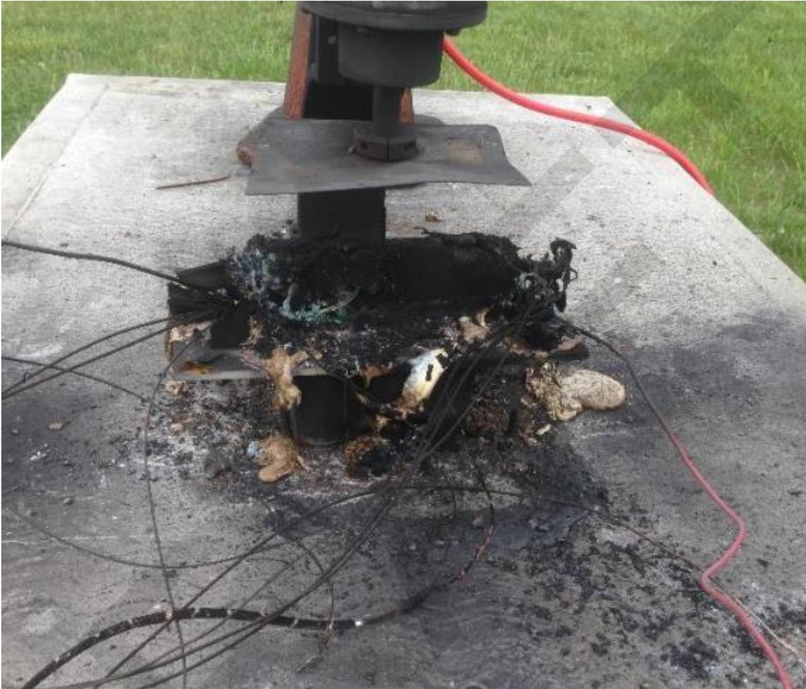
Figure 68. **PET – Nail Puncture Results 2**
