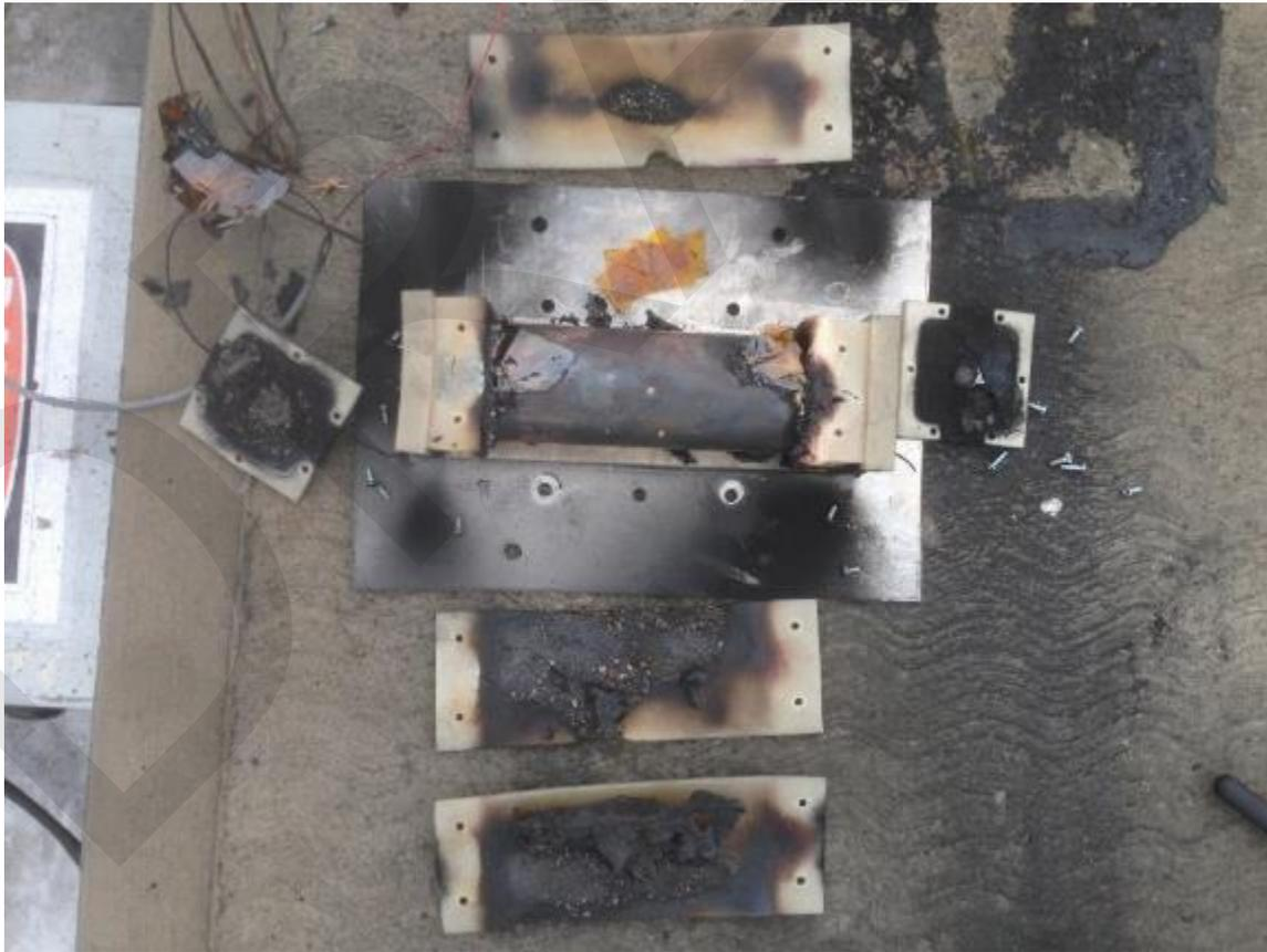
Figure 55. **Pyrophobic Material After Nail Puncture**
