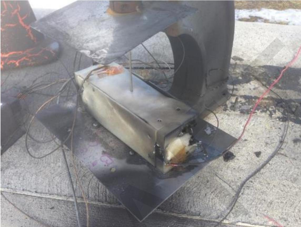
Figure 52. **Pyrophobic – Overcharge Results**
