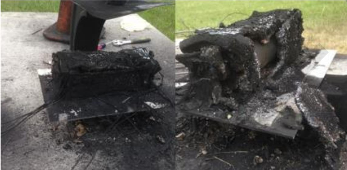
Figure 59. **Pyrophobic Overcharge with Enclosure Material Results**
