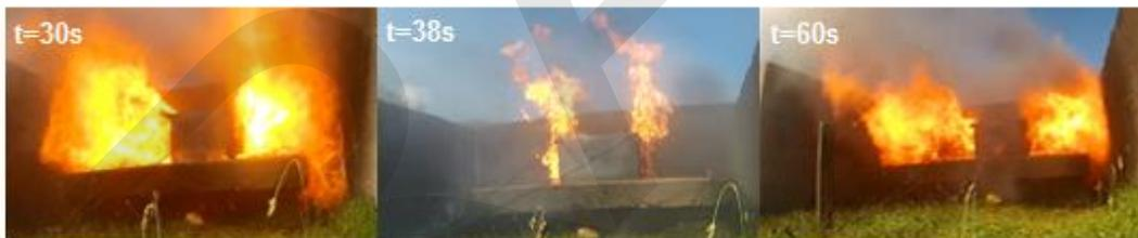
Figure 110. **Sequence of the venting process**
